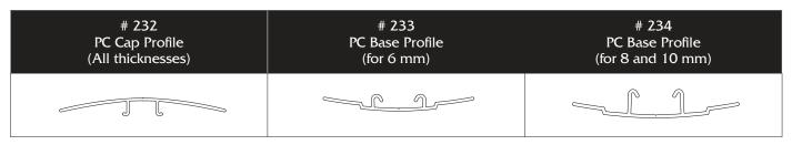
**GCP (Gasket Clip Profiles) connection profiles** with integrated gaskets are intended for use with sheets having a thickness from 6 to 10 mm sheets and are designed for greater water sealing capability. This system can be used in a wide variety of DIY, simple glazing and agricultural applications. The profiles have a "snap-and-click" design for connecting of base and cap profiles.
